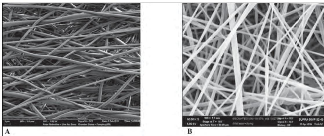
**Fig. 2** Microphotographs of CoPA fibers (a) and chitosan-based composite nanofibers containing chitin nanofibrils (b).
