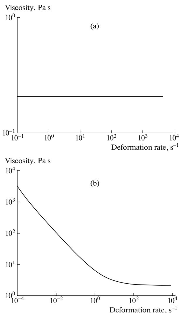
**Fig. 1.** Dependence of the effective viscosity  $\eta$  on the shear rate  $\dot{\gamma}$  for the copolyamide solution (a) and the mixture bearing 0.5% of SCNT (b).
