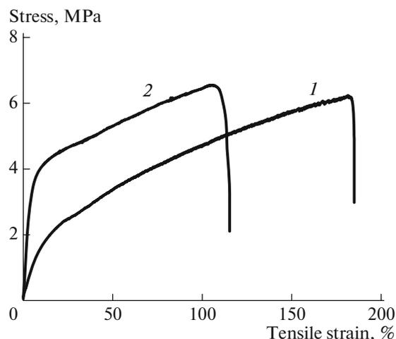
**Fig. 3.** Stress–strain diagrams for the film materials based on nanofibers from the copolyamide (1) and composite nanofibers bearing 0.8 wt % of SCNT (2).
