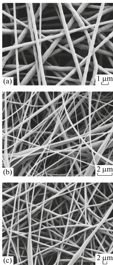
**Fig. 2.** Porous film materials based on composite nanofibers from the copolyamide bearing (a) 0.5, (b) 0.8, and (c) 2 wt % of SCNT.
